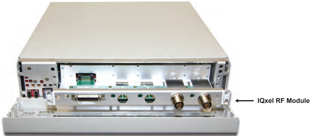
Figure 7: IQxel's Fully Calibrated, Replaceable RF Module
