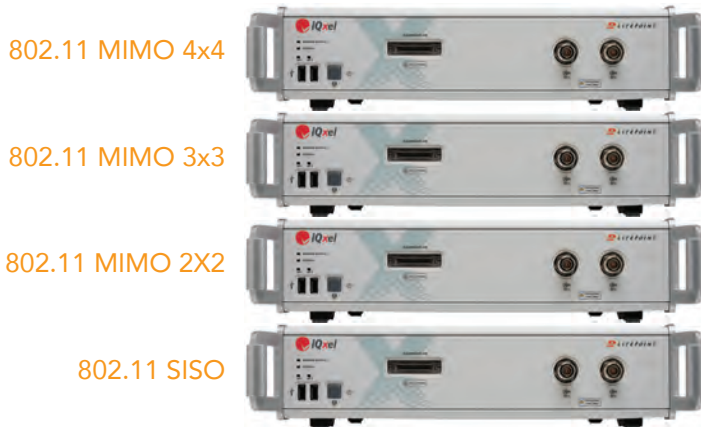
Figure 6: IQxel systems may be combined for MIMO applications as needed
