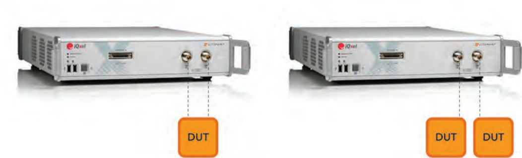
Figure 5a: IQxel160 testing an 80 MHz, 802.11ac, 2x2 MIMO device using True-MIMO method
