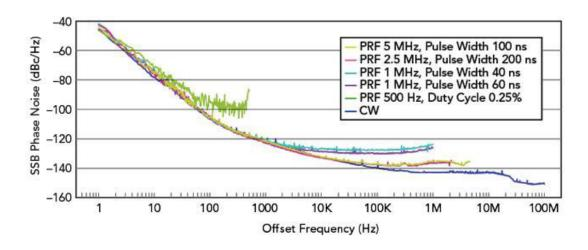
Figure 2 3.8 GHz pulsed signals, with pulse widths ≥40 ns and PRF ≤5 MHz.
