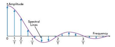
**Figure 1** Spectrum of a pulse modulated signal with pulse width  $\tau$  and pulse period T.
