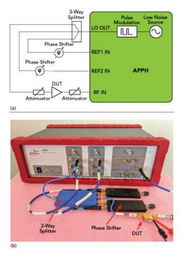
**Figure 3** Pulsed additive phase noise measurement using the internal LO of the APPH: block diagram (a) and photo (b) of the setup.
