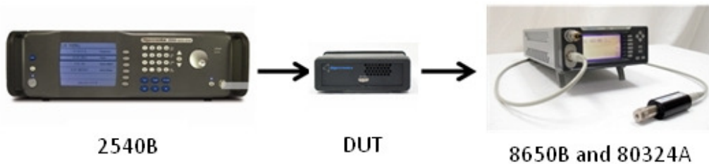
Figure 5: GT-1040A Performance Verification Setup
