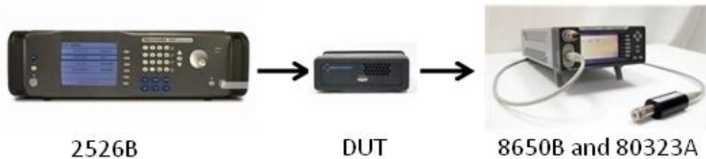
Figure 5: GT-1026A Performance Verification Setup
