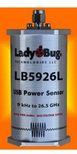
**LB5926L** is a state of the art high accuracy, high sensitivity True RMS Average power sensor. The sensor features frequency coverage down to 9kHz, making it ideal for source calibration and EMC testing applications. The Sensor's high damage level reduces source switching issues.
